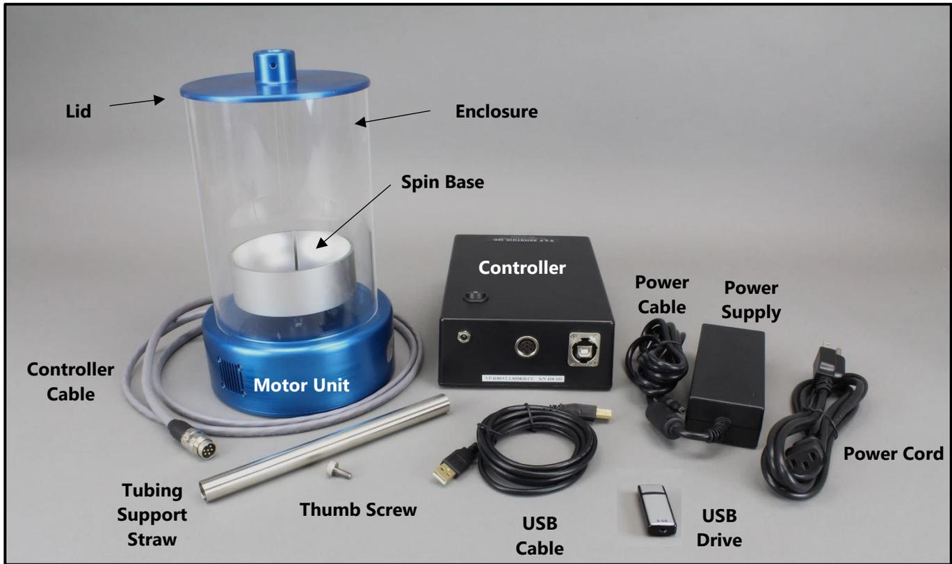
1. Connect the Power Cord from Power Supply to an outlet.
