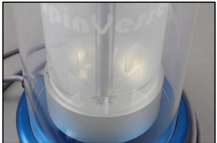
5. Insert the Tubing Support Straw into the hole in Lid and position it close to the bottom of the SpinVessel®. Tighten the thumb screw on the lid to hold the Support Straw in place.
