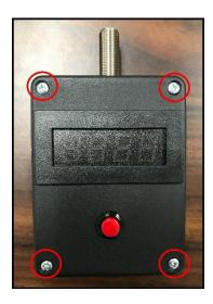
2. Gently remove the top panel to expose the inside of the RPM meter. The top panel is attached to the box, be careful not to pull any wires out of place. You will find the battery mounted to a white platform.
