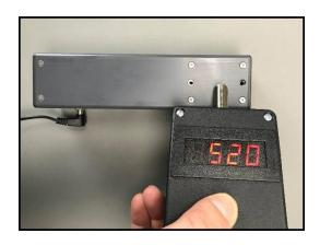
2. Ramp the tumble stirrer to the desired RPM. We recommend logging this position on the speed control knob. However you should be aware that if the load increases on the tumble stirrer motor the RPM count will decrease proportionately to the increased load. The reverse is also true, so it is wise to keep checking with the RPM meter and not totally relying on the speed knob position for accurate RPM determination.
