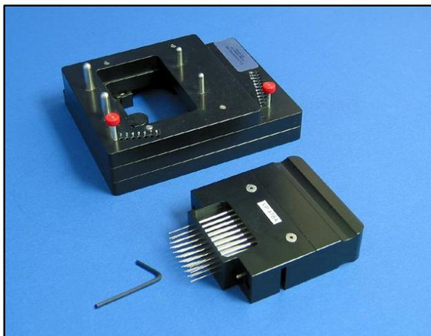
**Figure 1. Remove VP 478 or VP 478A Glass Slide Replicator from VP 470 Glass Slide Indexer and set on lab bench with Allen screws facing up.**
