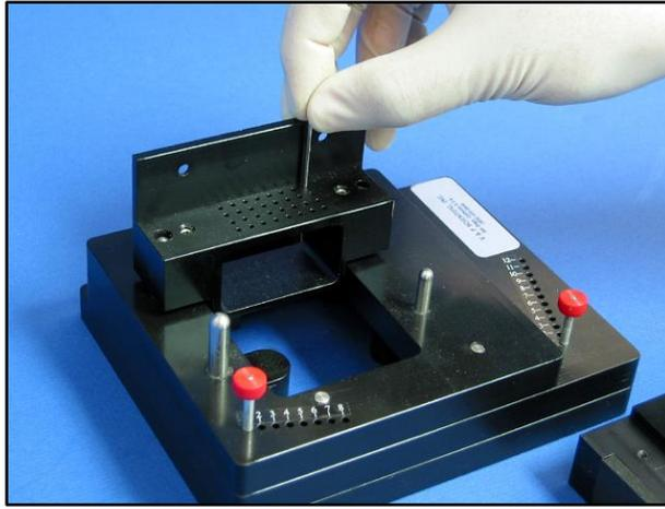
**Figure 4. Drop individual pins into upper pin hole. If pin does not drop directly through second hold, gently tap side of Glass Slide Replicator until pin drops in place.**
